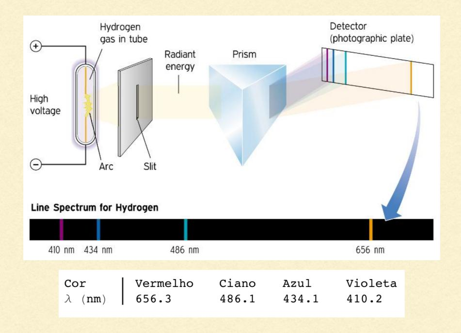
Signatures of a chemical element. This is how we know the sun is made of hydrogen.
