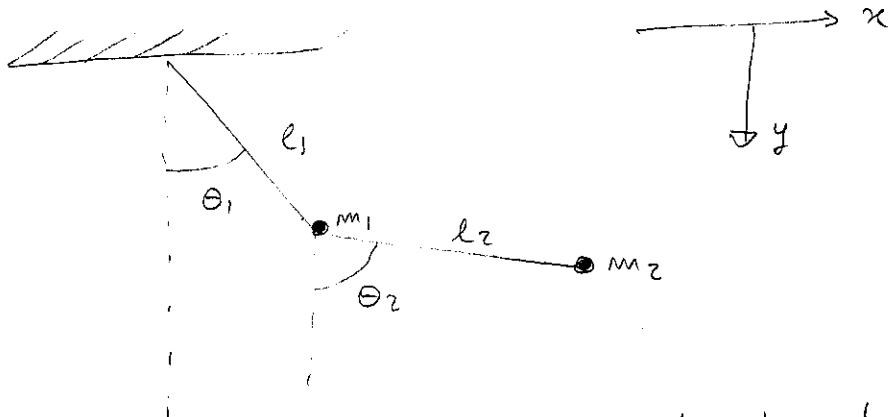
This is an important problem because it exhibits chaotic behavior. In principle there are 7 variables:  $x_1, y_1, x_2, y_2$ . But the masses are attached to the strings so we may completely describe the problem using the two angles,  $\theta_1$  and  $\theta_2$  (as defined in the figure).
