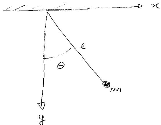
The position of the mass  $m$  is described by two coordinates :  $x$  and  $y$ . But it is silly to use two numbers since the length  $l$  is fixed. For this reason the position of the pendulum is completely characterized by the angle  $\theta$ . Based on my choice of coordinate system, we have
