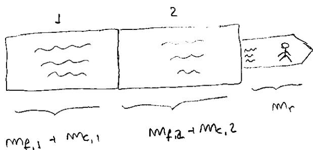
The part where the astronauts go is tiny and has mass  $m_r$ . Then there is a container with a bunch of fuel, the fuel weight  $m_{f,1}$  and the container weighs  $m_{c,1}$ . Similarly, there is another stage with  $m_{f,2}$  of fuel in a container with mass  $m_{c,2}$ . This drawing represents a 3-stage rocket.
