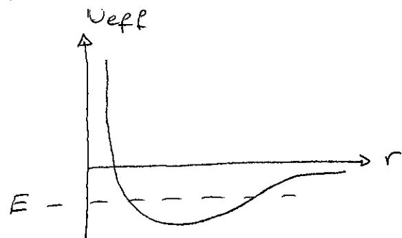
If (29) has only one solution  $r_{\min}$ , the motion will be infinite. This is what happens with comets, which approach our solar system, hang around for a while, and then leave.
