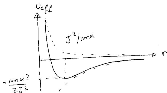
The gravitational interaction pulls the particle to the center while the centrifugal force pulls it away. This competition leads to a minimum, whose value is
