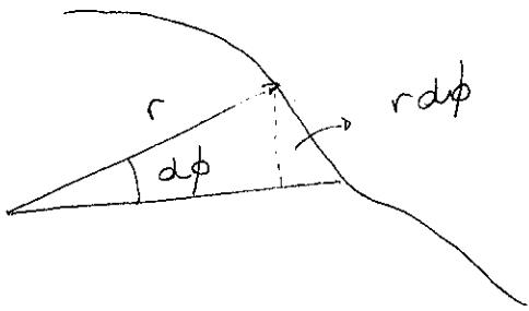
If we consider an infinitesimal chunk of the path, it has length  $r d\phi$  and therefore the banding area may be approximated by the area of a triangle:
