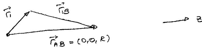
$$\vec{r}_{IB} = \vec{r}_{AB} - \vec{r}_A = -(x_1, y_1, z_1 - R)$$
