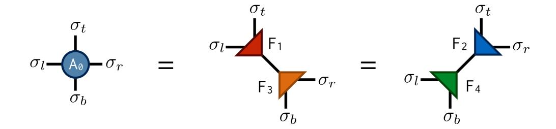
Each factorization can be derived from an SVD by grouping the square roots of singular values with unitary tensors:
