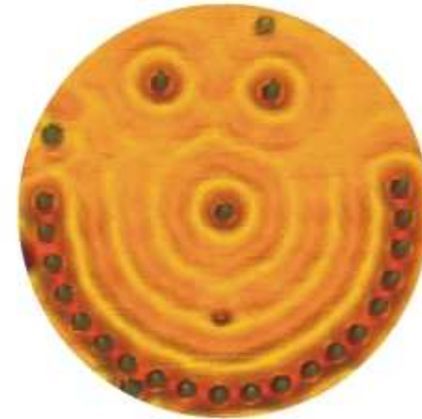
Ag atoms in a Ag(111) surface (STM). (Prof. Saw Hla's group, Ohio University)
