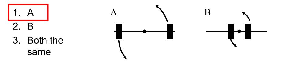
$I=\Sigma m_i (r_i)^2$  ( $r_i \rightarrow dist of particle$  "i" to axis)
